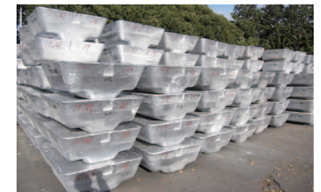
Can-to-Can aluminum recycling products. “Regenerated aluminum ingots”
