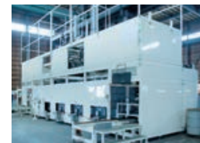
A cleaning machine for degreasing, washing, and drying of finely broken titanium scrap (Naoetsu Plant, Showa Metal Co., Ltd.).
