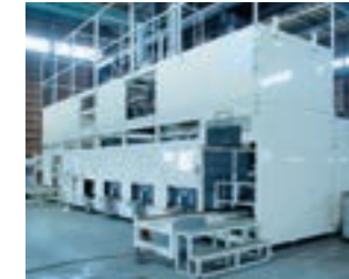
A cleaning machine for degreasing, washing, and drying of finely broken titanium scrap (Naoetsu Plant, Showa Metal Co., Ltd.)
