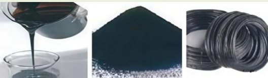
Pyrolysis-related products (from left: pyrolysis oil, carbon black, wire scrap)
